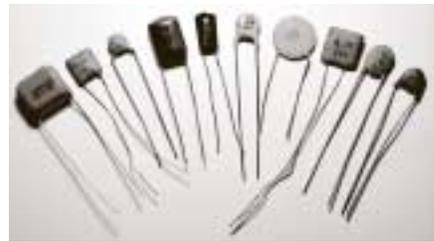
The value basically designates how much of the treble frequencies are shunted to ground when you roll
